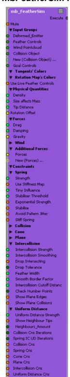
The mbFeatherSim node is by default located in the **Simulation stack**. It simulates the feathers' rotation with an unlimited amount of input forces and 4 predefined constraints. Stiffness, wind, gravity, collisions, intercollisions and many more featues are included in this node.
